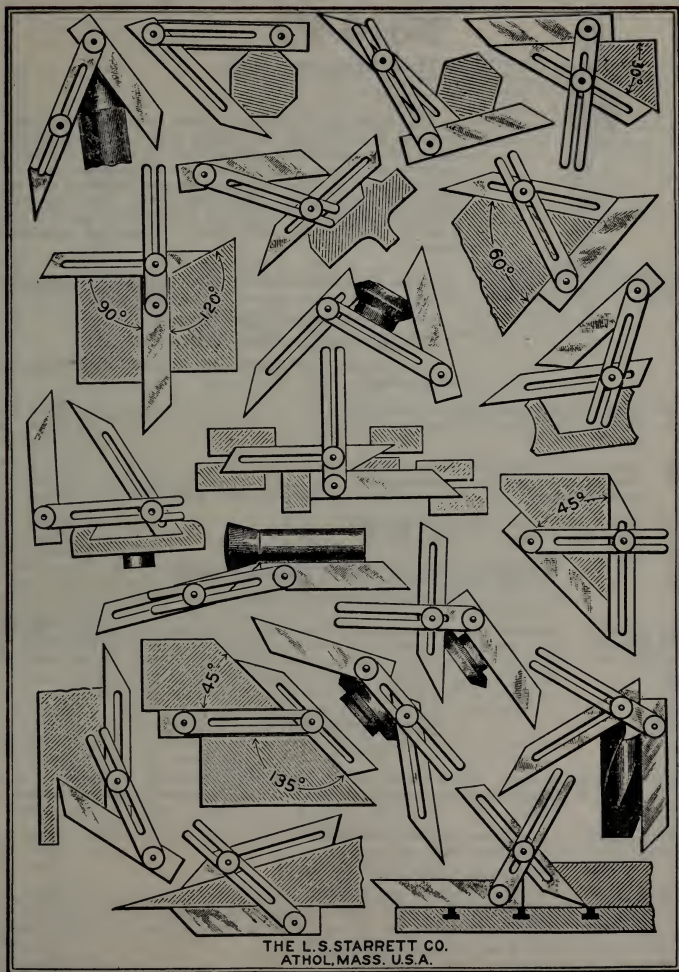
Showing some of the many uses of No. 49 Combination Bevel
